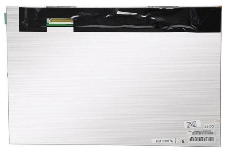
LCD Model B101AW06-V Active Area 222.72 (H) X125.28 (V) [mm] Pixels 1280 x 800 x 3(RGB) H x V Pixel Pitch 0.2175 (H)X0.2088 (V) [mm]
